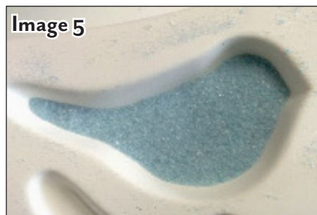
Fill the top sitting bird with F2 Alpine Blue Opal until roughly 1/4" full. If using fill weights, this is about 16 grams of frit.
