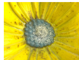
Fine frit shown obscuring the screw in the center of a frit casted flower.
