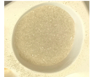
Add F2 Khaki until the cavity holds 20 grams of frit total.
