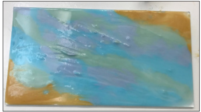
Image B: Frit slurries after initial blending with a plastic knife.
