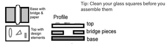
Apply a small dot of glue to the bridge pieces and place them on the base piece of glass aligned directly over each end of the base piece leaving a 1/4 " gap between the bridge pieces.
