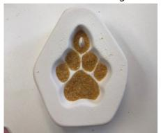
Put some F2 Medium Amber into the paw mold cavity. With a paint brush sweep the frit to expose the areas between the pads.
