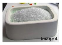
Once you're happy with your design, fill the remainder of the mold with Medium Clear. If using fill weights, fill until the total frit weight is about 250g. Before firing, gently sweep the frit away from the edges of the mold and mound it towards the center to avoid burrs (**Image 4**).
