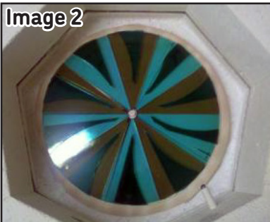
Image 2: Wedges of sheet glass arranged on Clear Iridescent atop Thin Fire Paper in the kiln.
