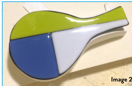
The fused glass on the mold before slumping
