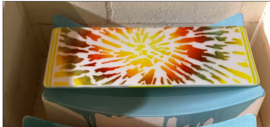
If you would like to slump your piece in the GM85 CPI Slump Mold , as pictured above, use the recommended firing schedule in Table 2 . (Treat the mold with a glass separator before firing.)
