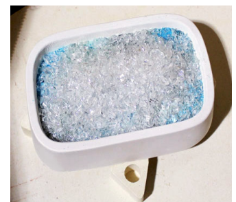
Image 12: Filled mold on kiln posts in the kiln
