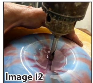
Image 12: Water lubrication via filling the flower's center with water
