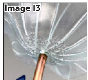
Image 13: 1/4" Copper Tube shown under 1/4" hole drilled in glass
