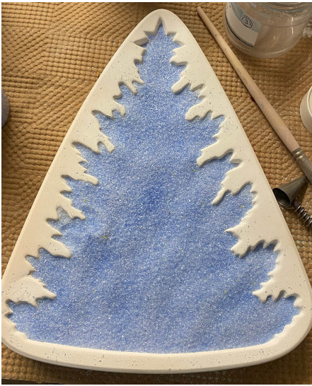
Step 3 Place a layer (approx. 1/4" deep) of Fine Pale Blue over the White in the mold cavity.
