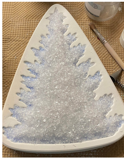
Step 4 Fill the mold with medium or coarse clear frit until the mold holds 425 grams of frit. Sweep the frit back to reveal the perimeter of the casting cavity
