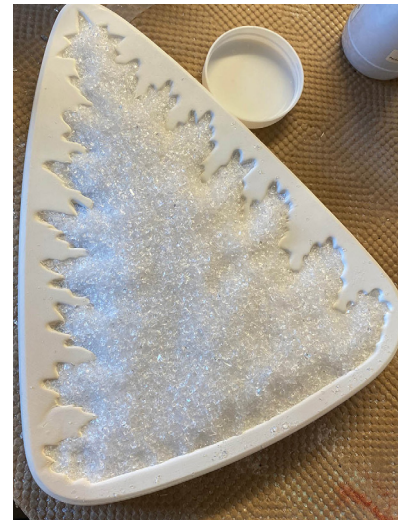
Step 9 Fill the mold with medium or coarse clear frit until the mold holds 425 grams of frit. Sweep the frit back to reveal the perimeter of the casting cavity.
