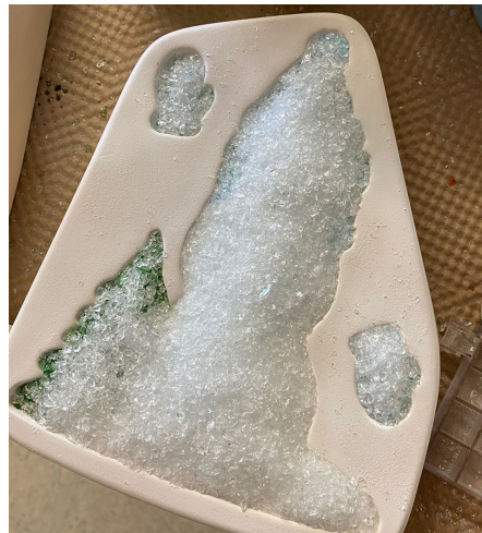
Back all of the frit with F3 Clear Frit until the mold is holding 175 grams of frit as shown above.
