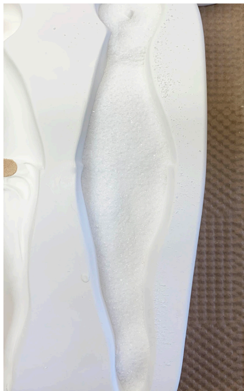
Place approx 1/4" white frit into the right Gnome.
