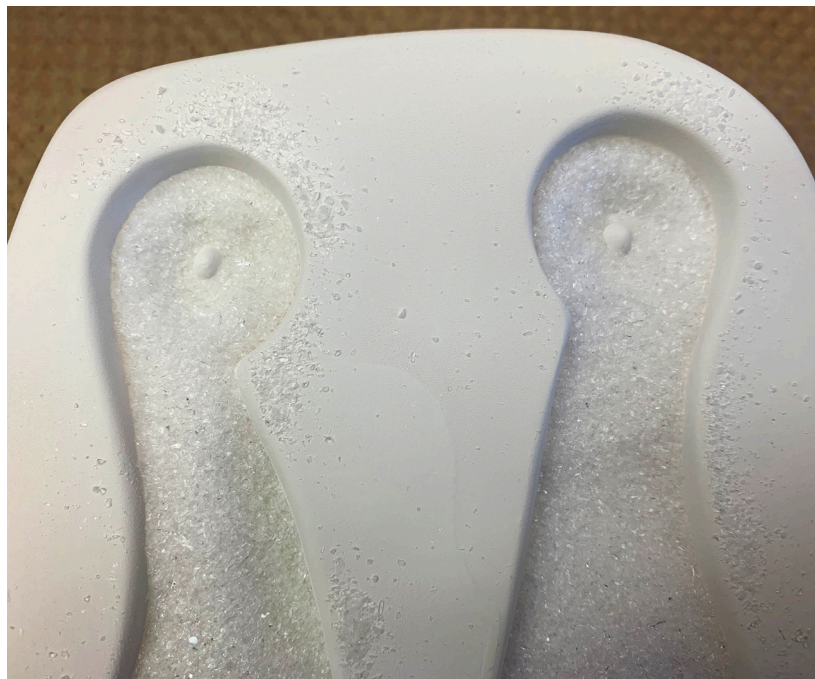
Use a tool or paint bursh to sweep frit away from the posts in the mold. Please read the Helpful Tips section on page 3 about removing the glass once it is fired.
