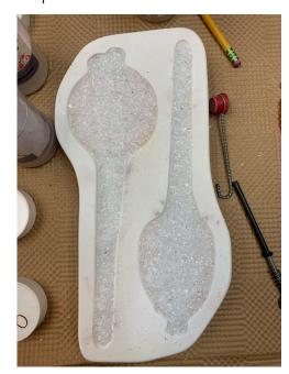
Back both pumpkins with F3 Clear until the total frit weight is around 305 grams (about 135g for the Thinner Pumpkin and 140 for the Wider). Place the mold in the kiln and fire to a Full Fuse using either our suggested schedule in **Table 1**, or your own preferred Full Fuse with a bubble squeeze.
