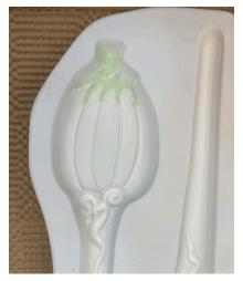
Begin with treating your mold with glass separator and allowing it plenty of time to dry (see Helpful Tips for more info). Once the separator is completely dry, begin by adding F1 Amazon Green to the top and bottom vines of the pumpkins.
