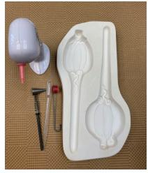
Here are our most frequently used tools for working with frit. In the top left is an Earwax Vacuum for precise frit removal. The three tools below it are (left to right) a Conical Sifter/Line and Dot Sifter, a plastic Eyedropper with the bulb cut diagonally to create a scoop, and an Enamel Sifter.
