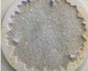
Fill the mold with medium grain and or coarse Clear frit such that the mold is holding 345 grams of glass. suggested schedule can be found in Table I.
