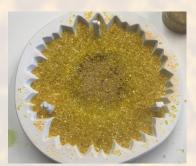
Cover the petal area of the mold with a layer of medium grain Yellow Trans frit, such that all of raised area of the mold is now covered with frit. Spread some of Fire the project using your the Yellow Trans frit into the seed favorite full fuse schedule. A area as well.
