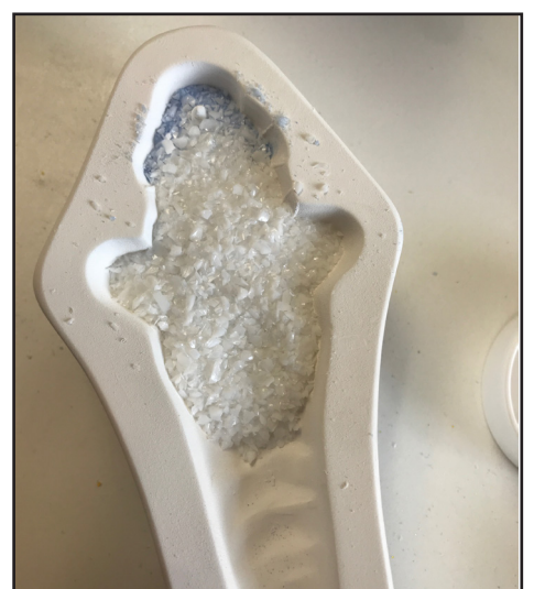
Back the entire snowman portion of the mold with F3 White.
