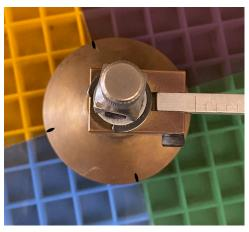
Place a circle cutter set to cut a 12.75" circle on the glass such that the marks on the suction cup are over the seams between the glass colors. Hold the center of the circle cutter tightly in place and
