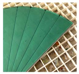
Use Pattern 1 and a marker to mark each quarter circle into 8 equal parts. Use a straight edge to score from the outside mark to the point of the quarter circle. Begin with the center line and break it away to create two pieces and then score
